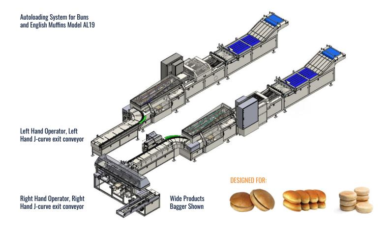
LMC's AL19 has a mechanically distributed drive train connecting all conveyors, baggers, and slicer belts to give reliability and consistency like a classic autoloader. It also features a redundant motor starter drive, parallel to the VFD, geared for 60 bags per minute. Precision aligned, fixture welded frame. Matched safety sensors and integrated safety PLC, Cat3. Long-life top transfer guaranteed thanks to its CNC parts and an aligned frame.
