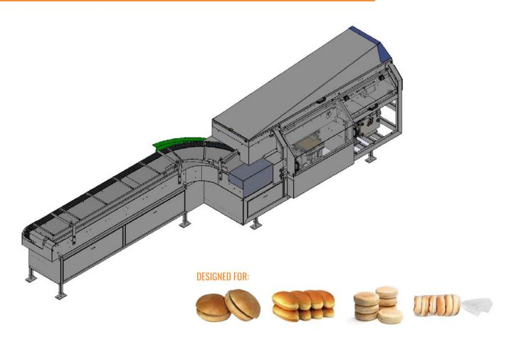
LMC's HL18 is a bagging machine that pairs with a packing conveyor. Geared for 60 bags per minute. This allows an operator to load products into the flighted infeed of the bagger. It has a mechanically distributed drive train connecting all conveyors and chain to give reliability and consistency. Precision aligned, fixture welded frame. Matched safety sensors and integrated safety PLC. CAT3 safety rated. Long-life top transfer guaranteed thanks to its CNC parts and an aligned frame.
